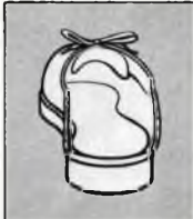
Here is a cutaway picture of an ordinary shoe heel. You will notice that the heel seat is nearly flat—not cupped to take the rounded heel of a foot. To keep the weight line straight, a shoe should hold the heel firmly in a supporting grip.
