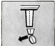
This is a weak table leg. The weight line down the center is not straight—sit on the corner of this table and the leg rolls inward.
